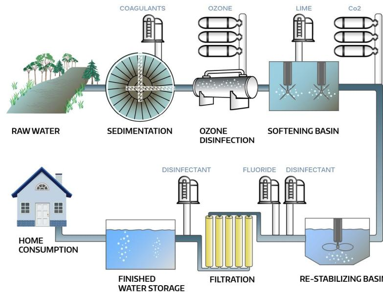
Raw water is drawn from our fresh water sources - the Kansas and Missouri Rivers, adjacent collector wells, and conventional wells on the Kansas River - and collects in our pre-sedimentation holding basins. Water then goes through the following stages as part of the treatment process.
