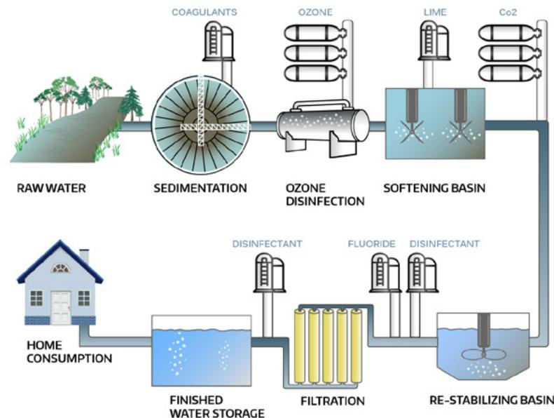
Raw water is drawn from our fresh water sources - the Kansas and Missouri Rivers, adjacent collector wells, and conventional wells on the Kansas River - and collects in our pre-sedimentation holding basins. Water then goes through the following stages as part of the treatment process.
